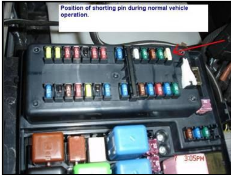
Toyota Land Cruiser fuse box with the shorting pin identified in Normal Vehicle Operation Mode
