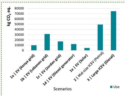
**Figure 11:** LCA results for global warming for production, use (200,000 km), and disposal
