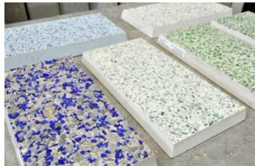
(b) Architectural concrete using waste glass
