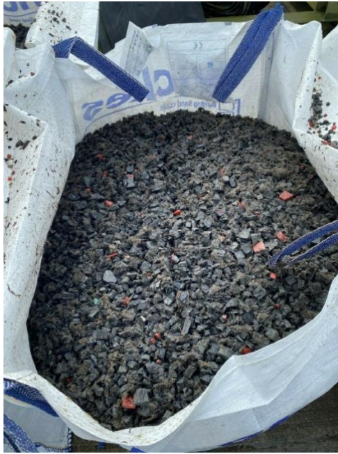
Figure: Shredded rubber from used tires stored in sacks
