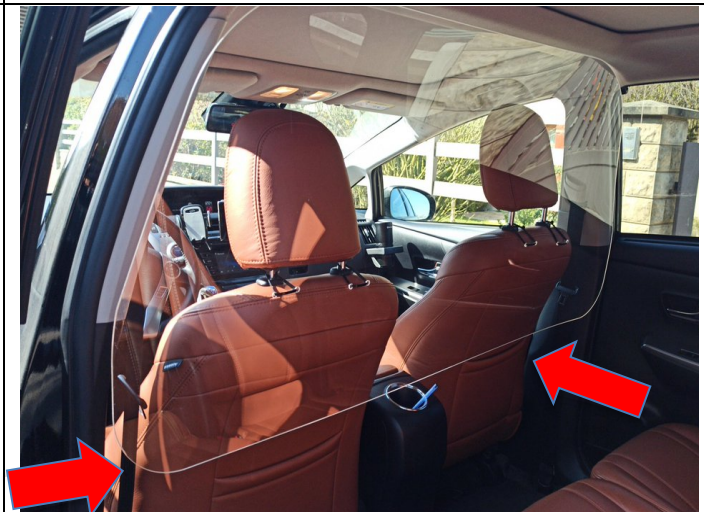
Partition in plexiglass, not waterproof; the vehicle is considered as not equipped of partition
